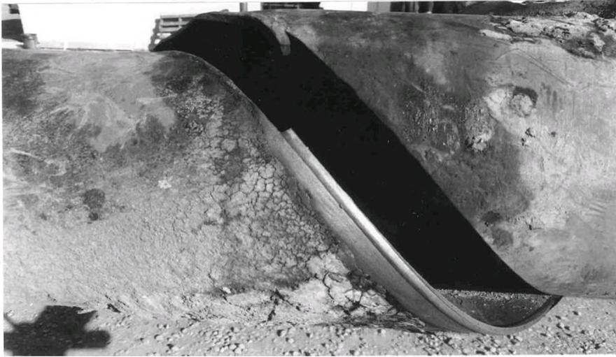
Failure of spirally-welded pipeline from Stress Orientated Hydrogen Induced Cracking.
